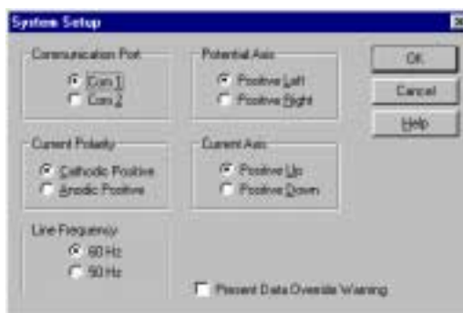
System setup allows any convention of current and potential polarity.
