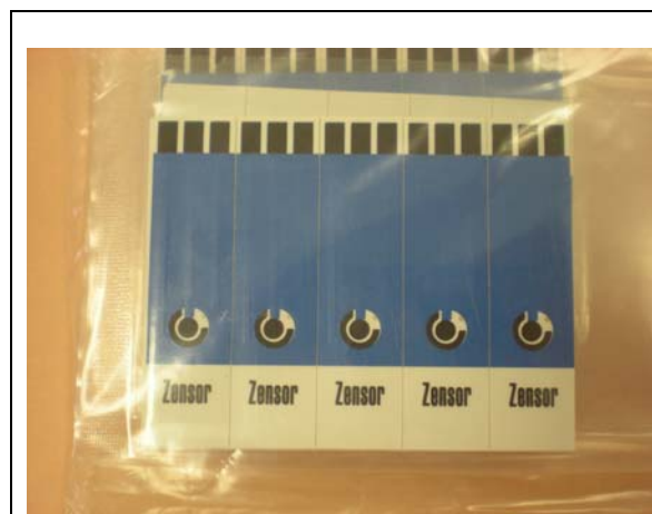
TE100: three electrodes with 3mm diameter working electrode.
