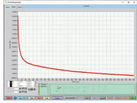
Fig. 3-1. Amperometric i-t curve of 2 mM potassium ferrocyanide during electrolysis at constant potential.
