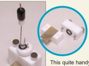
This quite handy cell was developed in order to evaluate a plate material such as metal, semi-conducting plate, etc.
