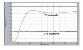
The light transmittance was compared with ITO electrode and Grid electrode (Au, Pt and Carbon) on a quartz glass as a reference. For ITO electrode the light cannot be transmitted easily in an ultraviolet range. The transmittance is about 10% at 280 nm of the wavelength. For wavelength above 400 nm the transmittance is above 80%. Compared with the quartz glass, the light transmission for grid electrode is about 30%, however it could be used in an ultraviolet range.
