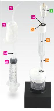
RHE is a reversible electrode kit, in which hydrogen gas is generated by electrolysis of strong acid then stored. It makes unnecessary the complicated and dangerous set-up of the hydrogen cylinder and avoids the large volume of hydrogen gas exhaustion, despite that it has a good potential stability.
