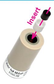
Disk Replaceable Electrode (DRE) has a removable disk electrode. The replacement of the disk electrode is possible from both side, front side and rear side. It makes possible to choose, according to the condition required for your research purpose.
