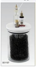
Bulk electrolysis cell is used for complete electrolysis of solution. Typical application includes quantification of mass transfer of the electron per molecule, measurement of absolute quantity of the analyte, electrolytic synthesis of new materials (generally in quantity of milligram).
