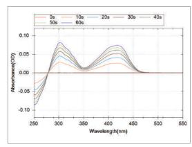
Fig. 3-2. Time course of absorption spectrum during the oxidative electrolysis of 2 mM potassium ferrocyanide.
