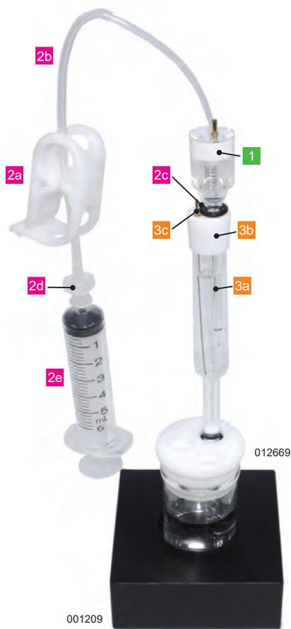
RHE is a reversible electrode kit, in which hydrogen gas is generated by electrolysis of strong acid then stored. It makes unnecessary the complicated and dangerous set-up of the hydrogen cylinder and avoids the large volume of hydrogen gas exhaustion, despite that it has a good potential stability.
