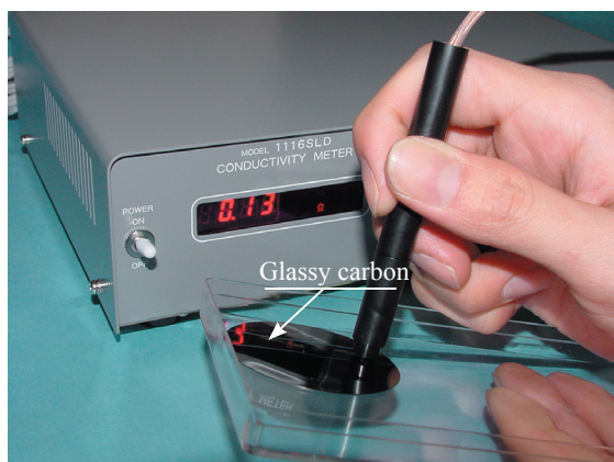
Figure 9. Resistance of Glassy carbon thin plate is measured by contact probe.
