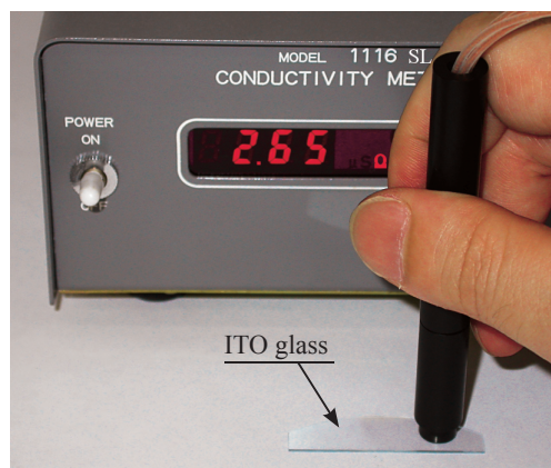
Figure 10. Resistance of ITO glass plate is measured by contact probe.
